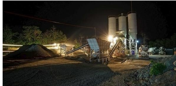
**NIGHT POURING AT TPLEX PROJECT.** *The state-of-the-art wet-mix concrete batch plant of Ten-Four Readymix Concrete, Inc. at Rosario, La Union produces high performance concrete using **Magnus 700G** to be poured at the TPLEX Project.*
